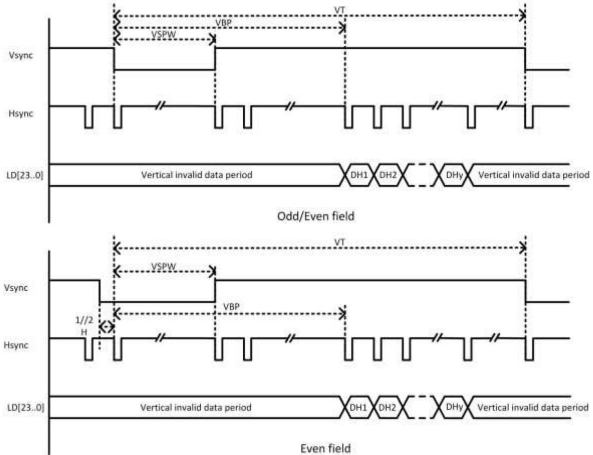
Figure 5-9 HV\_IF Interface Horizontal Timing
