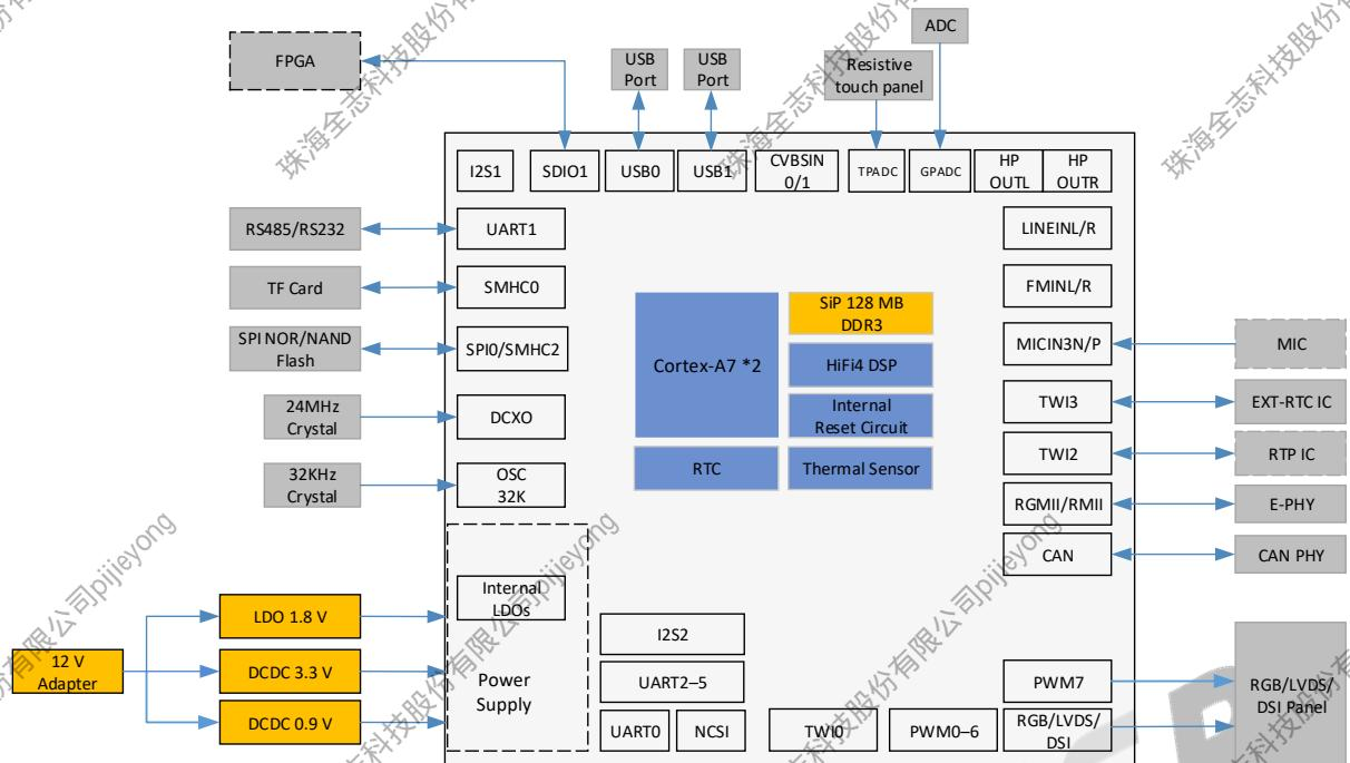
**Figure 3-5 Industrial Control PLC Solution of the T113-S3**
