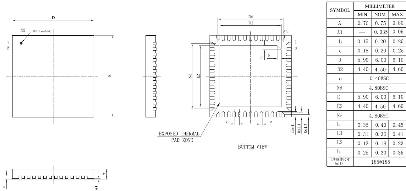
Figure 4-2 QFN52 Package Outline Drawing
