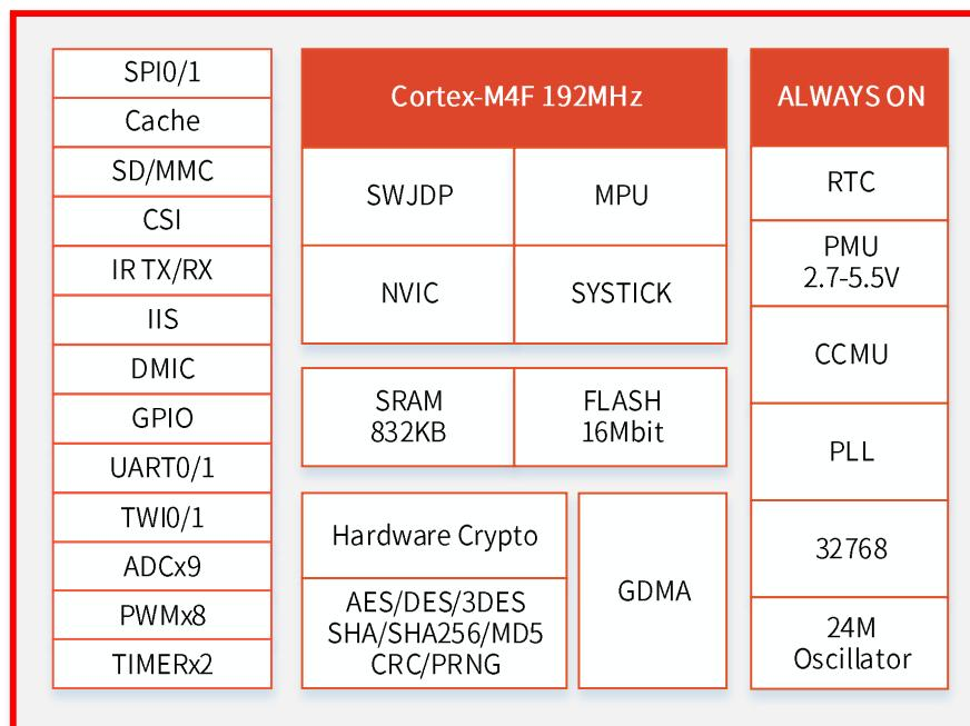
Figure 1-1 XR32F429 Functional Block Diagram
