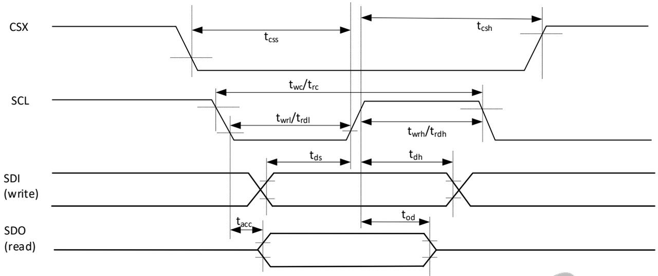
Table 5-25 DBI 3-line Serial Interface Timing Parameters
