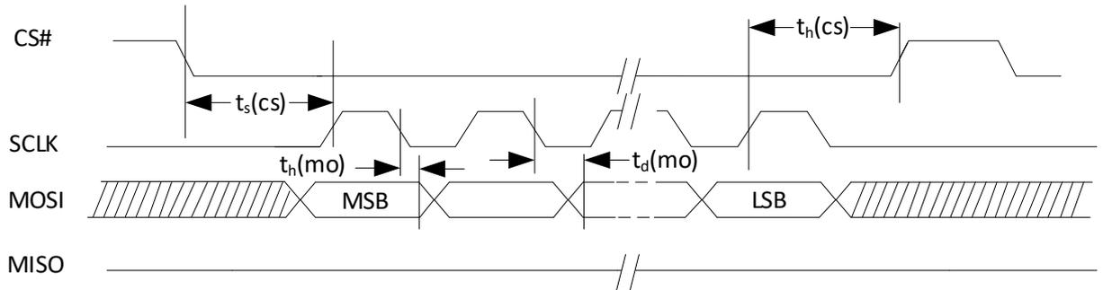
Figure 5-16 SPI Reading Timing
