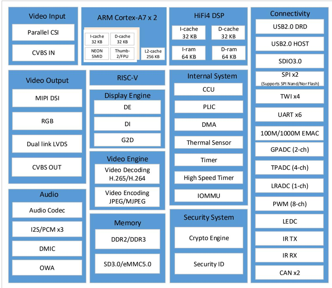
Figure 3-2 shows the solution of T113-i multi-media decoding platform.
