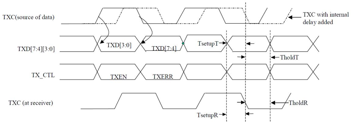
**Figure 5-14 RGMII Interface Receive Timing**
