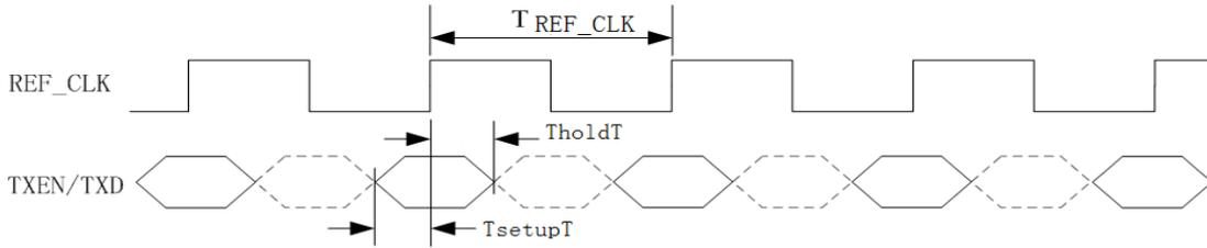
Figure 5-12 RMII Interface Receive Timing
