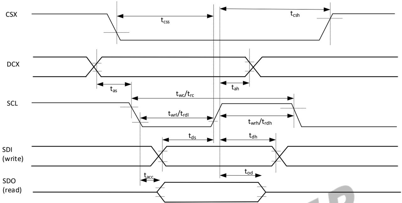
**Table 5-26 DBI 4-line Serial Interface Timing Parameters**
