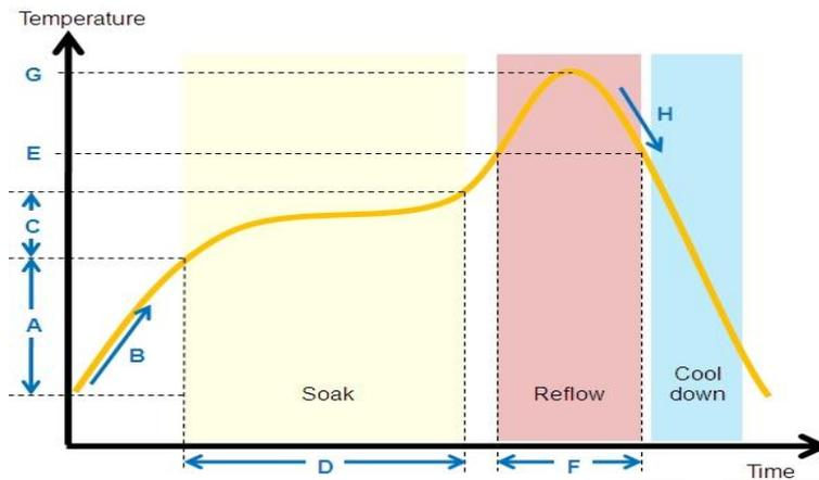
Reflow profile conditions of AXP2101 device sample is given in Table 9-1.
